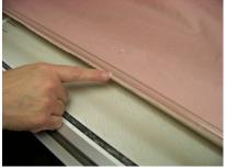
At the front of the machine, clamp the backing leader over the stabilizer bar on each side to hold it in place.
